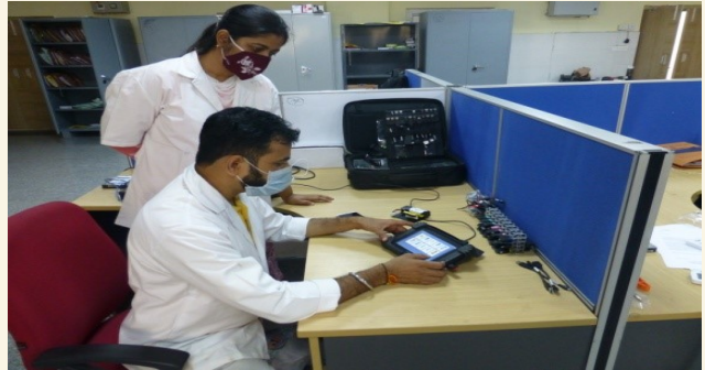
UFED TOUCH SYSTEM (ANALYSIS AND RECOVERY OF DATA FROM DIGITAL EVIDENCE)
