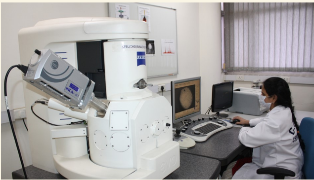
SEM-EDXA SYSTEM (SCANNING ELECTRON MICROSCOPY (SEM) WITH ENERGY DISPERSIVE X-RAY ANALYSIS)
